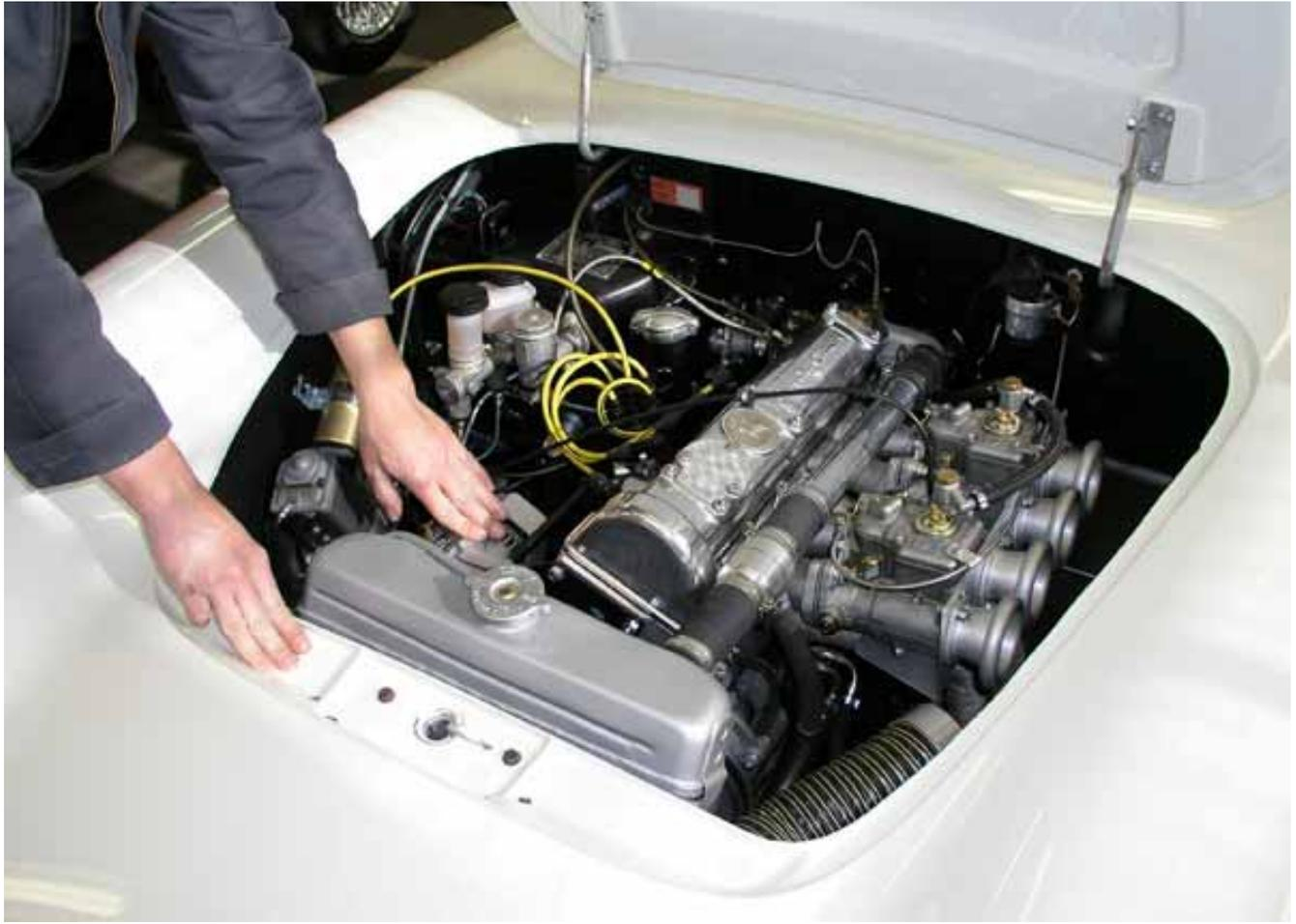
Though we planned to duct intake air to the carbs I did an initial road test without a duct and found engine bay temperature at the intakes was rarely below 40 deg C and climbed past 60 deg C when stopped and idling in 20 deg C ambient. With the addition of a 3-inch duct from in front of the radiator to the trumpets temperature rarely rose beyond 40 deg C, and declined quickly to near ambient at speed.
