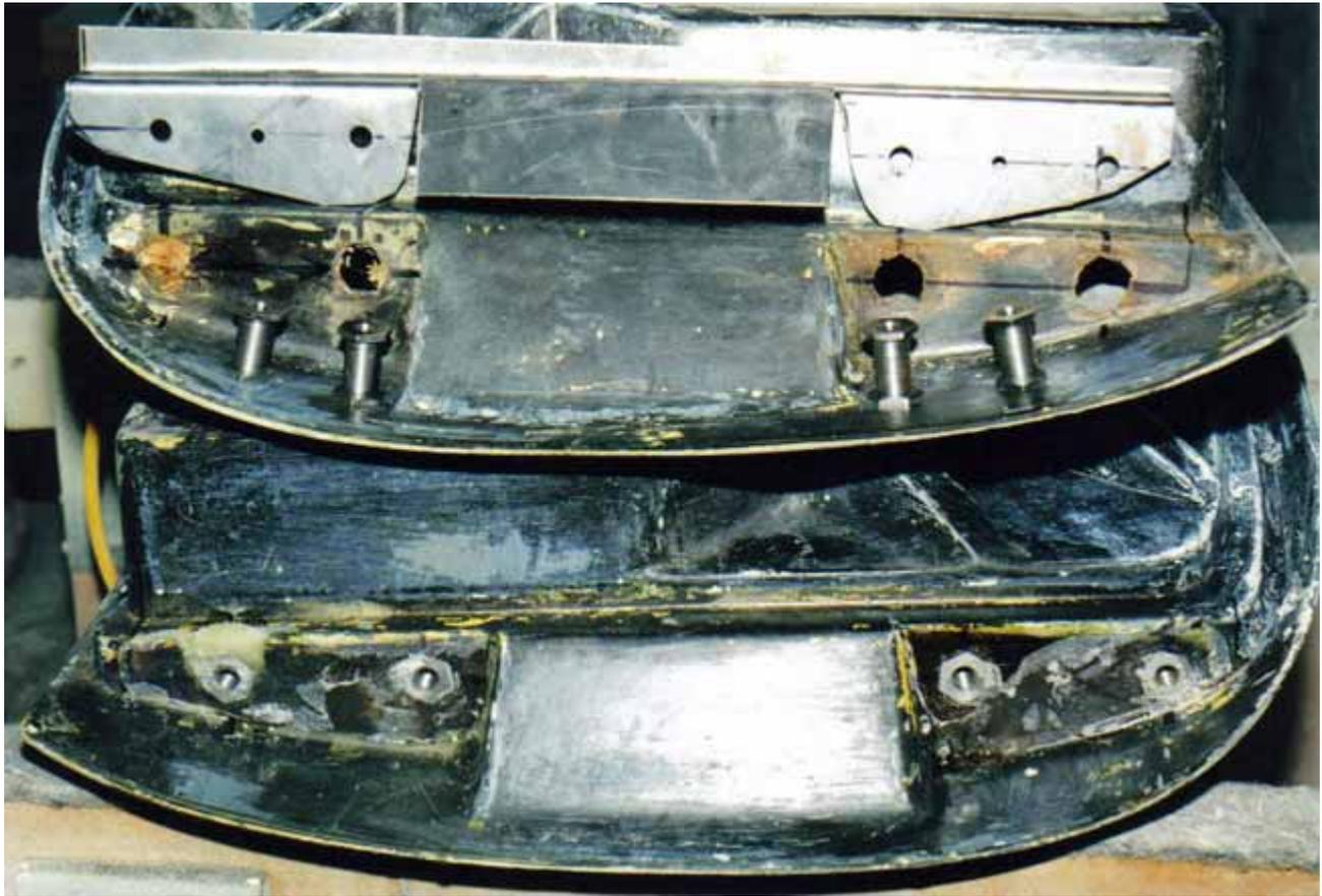
Top door: original bobbins torn out, new bobbins and their positions marked and sheet metal jig ready for location. Bottom door: new bobbins bonded in.
