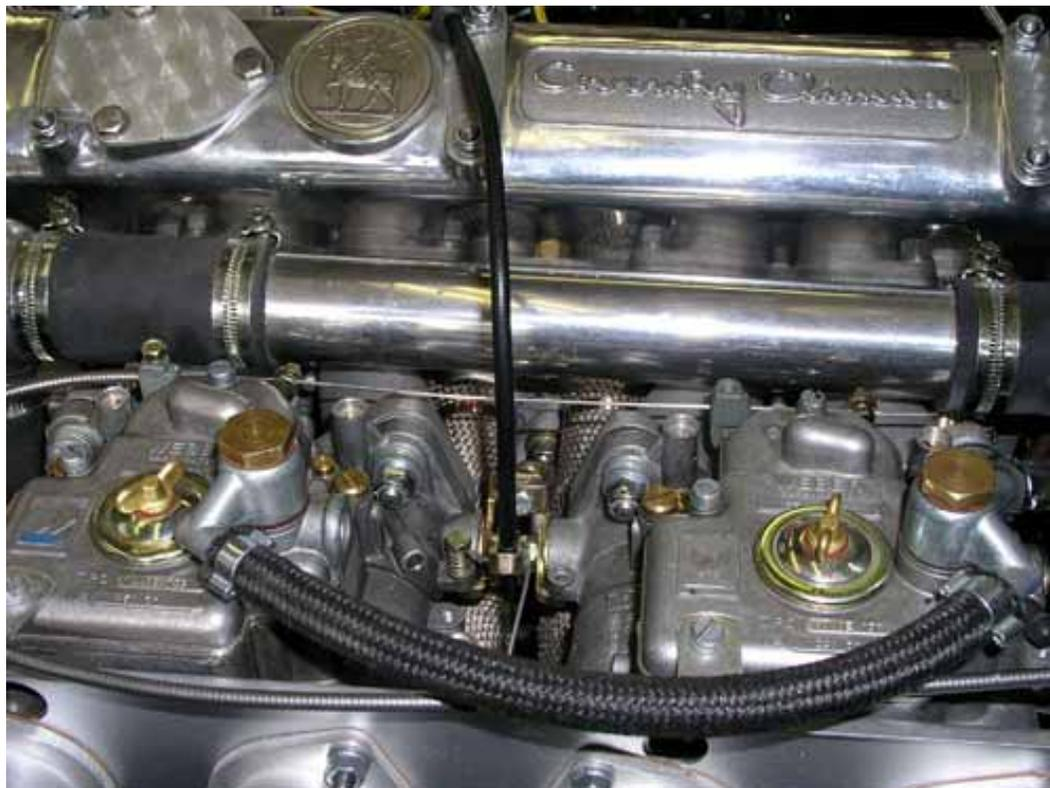
The original throttle pedal for SUs needed its lever extended to obtain enough cable stroke at the carb levers. A hairpin return spring like the one on Elan Webers was made from piano wire.
