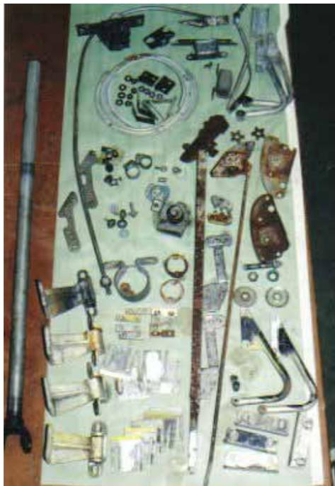
Many of the steel body and mechanical parts and fasteners were originally plated with silver cadmium or zinc. These were all stripped and re-plated. For racing we substituted aircraft-grade fasteners in the suspension assemblies.
