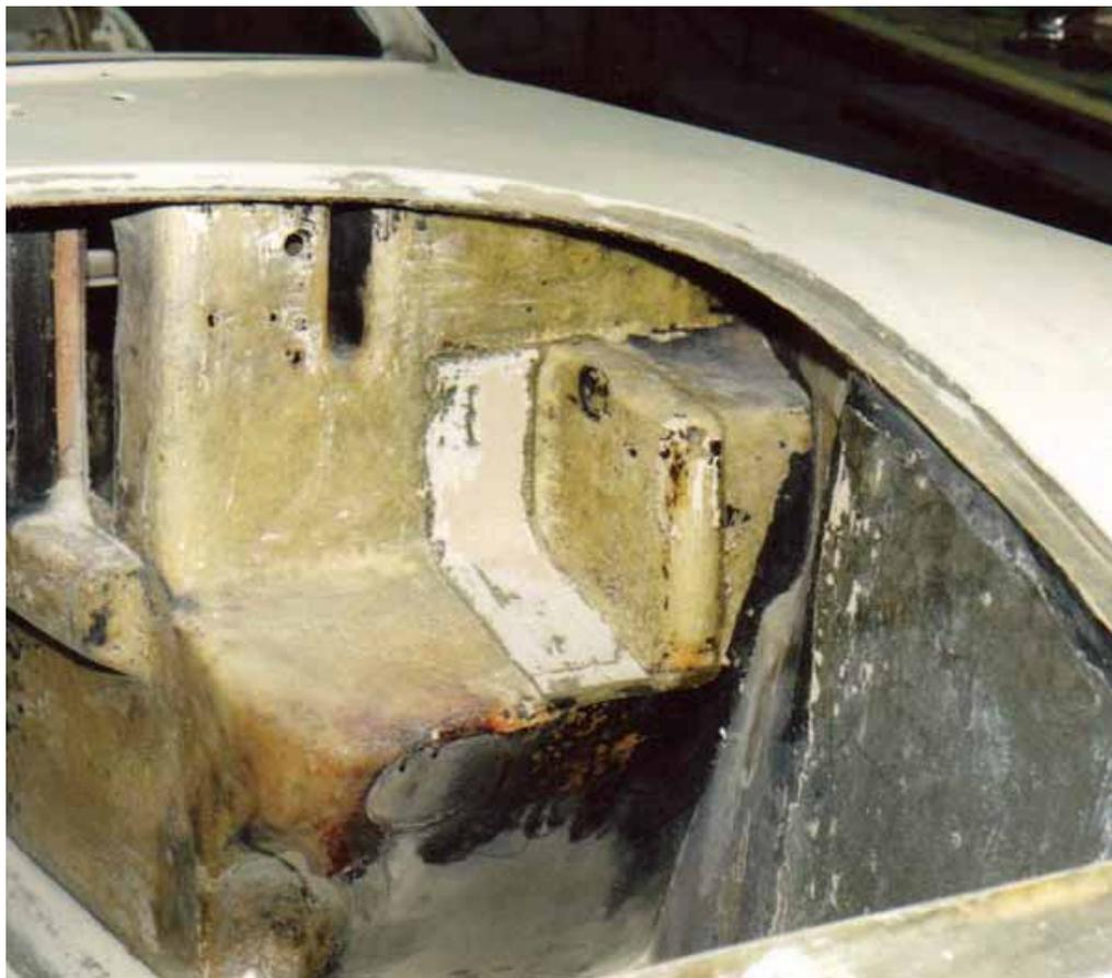
Pieces bonded from the inside, ready for filling & sanding. Note resin above starter blister is cooked red/brown from exhaust.
