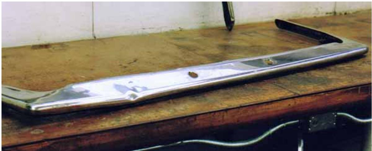
I have not been able to find a reliable metal finisher who is patient enough to massage these delicate hand-made pieces back into shape, so I have spent many hours learning and practicing. The flat expanse on the rear bumper is especially challenging since the slightest distortion is plainly visible. With great patience and various steel dollies, wood blocks, rubber mallets, files and felt marking pens the
