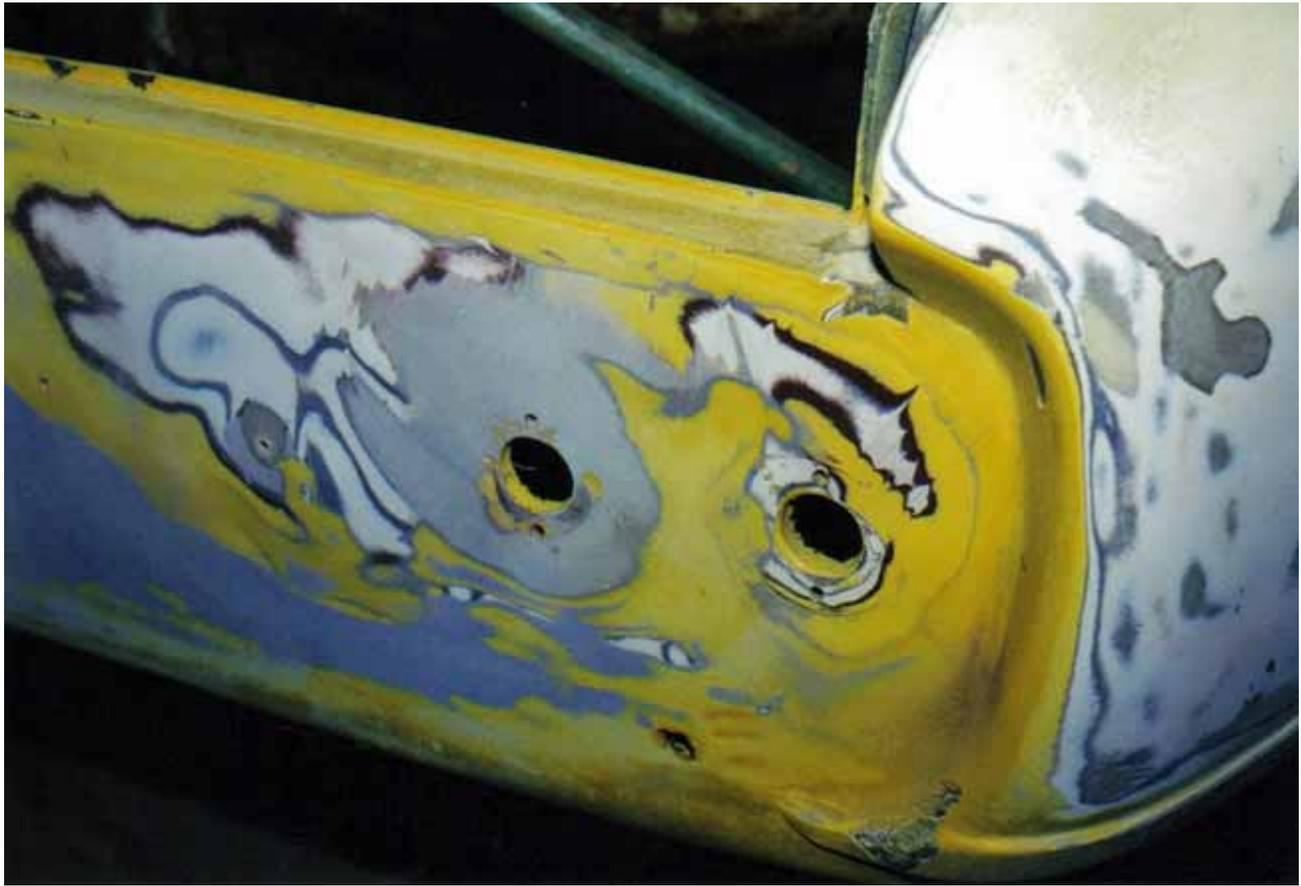
Paint stripping. Two yellow and one white respray with associated primers and fillers on top of original white.
