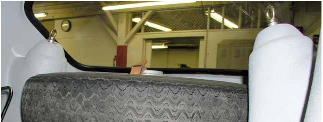
To anchor the shoulder harness we devised an extended rear strut top nut.
